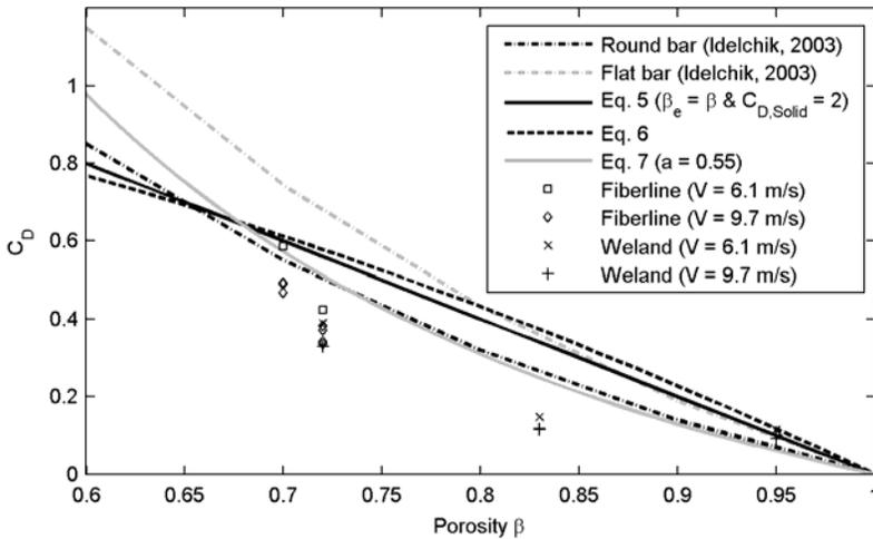
**Figure 4.** Measured drag coefficients for the different gratings.
