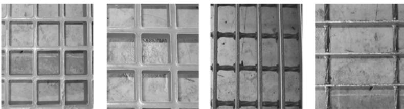
**Figure 2.** Pictures of the four grates used. From left to right is Fiberline 40, Fiberline 50, Weland H4 and Weland J9. The pictures are taken so the grates are viewed from the bottom (the side facing the jet).
