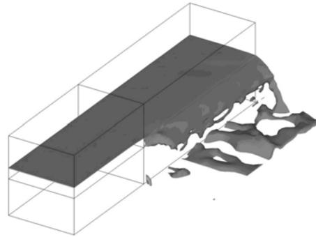
Figure 6 Numerical model of side weir
