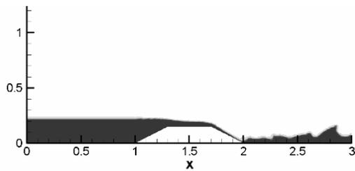
Figure 3 Computation with NS3 of flow over broad-crested overflow
