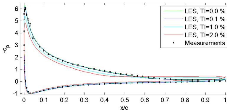
Figure 3: Pressure coefficient for  $14^\circ$  angle of attack
