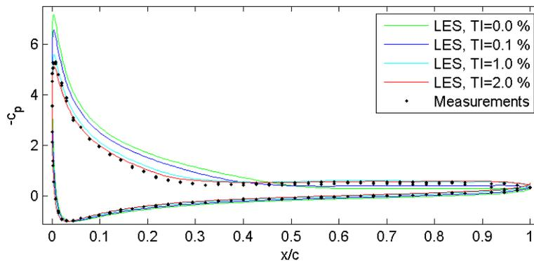
Figure 4: Pressure coefficient for  $16^\circ$  angle of attack
