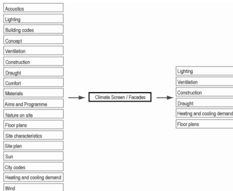
Figure 2 Example of the interaction of the parameters in the Integrated Design Process, when sketching on the climate screen.
