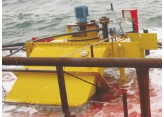
Figure 9: Kaplan turbine with Siphon inlet
