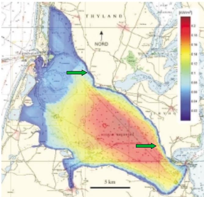
Figure 3: Energy density in Nissum Bredning. The figure also shows the 2 different locations where the machine will be placed.
