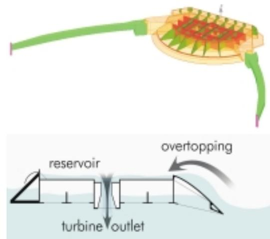
Figure 4: The Basic principle of the Wave Dragon.
