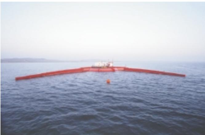
Figure 1: The Wave Dragon Nissum Bredning Prototype.
