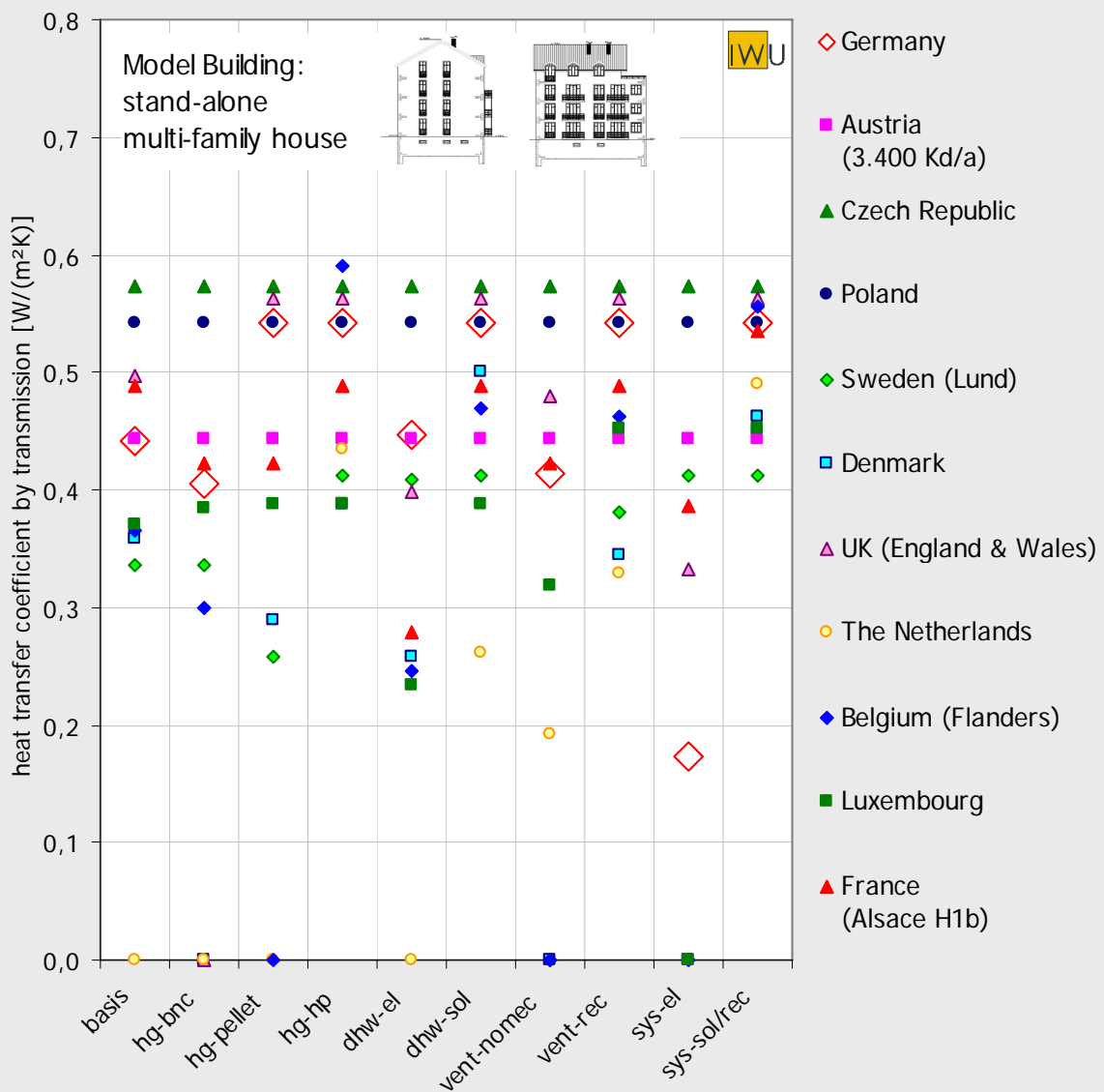
Fig. 5: Results for Model Building 2 (multi-family house) – simplified heat transfer coefficient by transmission (zero = requirements can not be complied, “-“ in Tab. 8)
