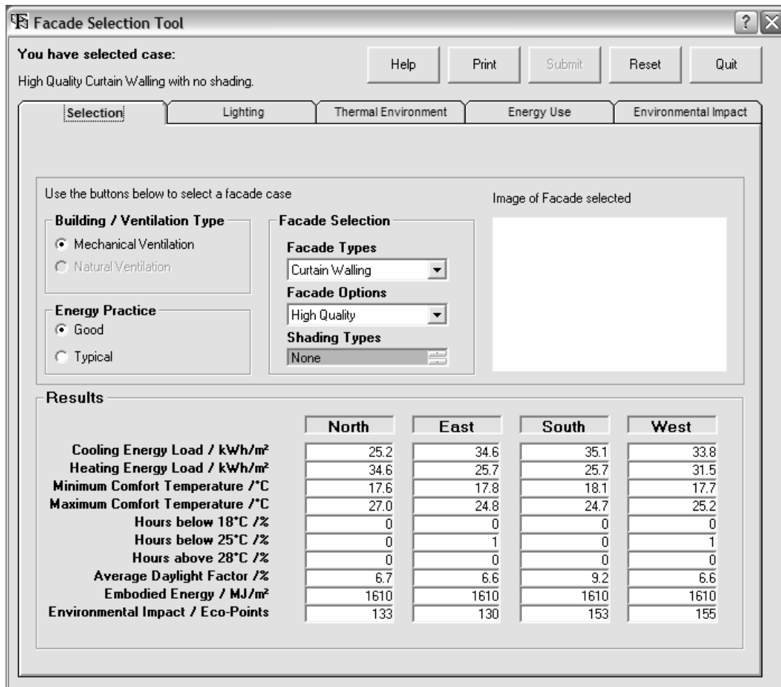
Initial screen of the Tool indicating the required input and presenting summary outputs.
