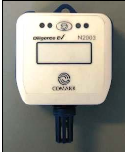
Figure 45. COMARK data logger N2003.
