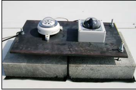
Figure 40. Photo of pyranometers on the roof of 'the Cube', Wilhelm Lambrecht pyranometer at the left and BF3 at the right.
