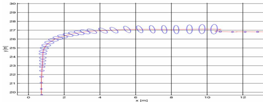
**Figure 4:** Navigation field tests. The GPS measurement update is omitted from point (0.7, 20), but the filter maintains an estimate to the position. The ellipse indicates the covariance of the state estimate.
