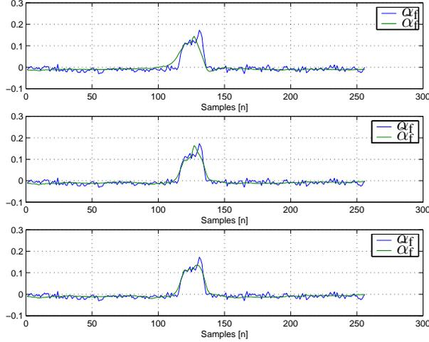
Fig. 2. Illustration of the Karhunen-Loève approximation of  $\alpha_f$  which contain a typical scratch. The first approximation is based on the one most approximating coefficient, the second approximation is based on the five most approximating coefficients, and the third approximation on the seven most approximating coefficient.
