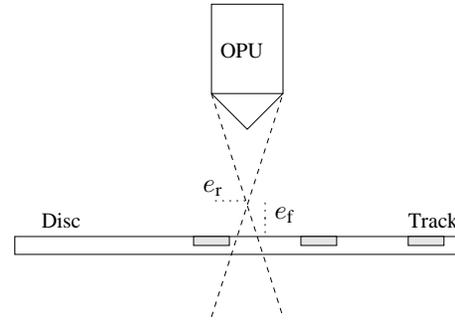
Fig. 1. The focus error  $e_f$  is the distance from the focus point of the laser beam to the reflection layer of the disc, the radial error is the distance from the centre of the laser beam to the centre of the track. The OPU emits the laser beam towards the disc surface and computes indirect measurements of  $e_f$  and  $e_r$  based on the received reflected light. In addition the OPU generates two residuals which can be used to detect surface defects as scratches.
