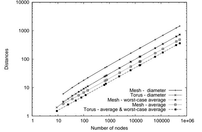
**Figure 2. Distances in non-hierarchical mesh and torus structures.**
