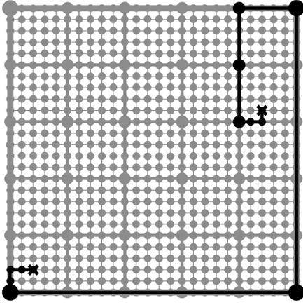
**Figure 1. The perfect square mesh with  $g = 5$  and  $n_H = 2$ . It is indicated how the distance between the two marked nodes has been reduced from 34 to 12 by hierarchical lines.**
