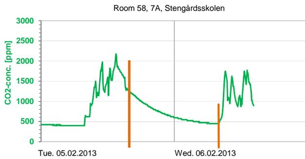
Figure 6. CO<sub>2</sub>-concentration. Orange lines indicate a period where the room is considered unoccupied
