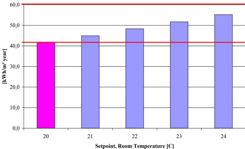
Figure 4 Total energy demand of a standard house with different setpoints of the room temperature, calculated according to the energy frame of Danish Building Regulation 2008. *Low Energy Class 1* is 42.1 W/m<sup>2</sup>K year and *Low Energy Class 2* is 60.4 W/m<sup>2</sup>K/year
