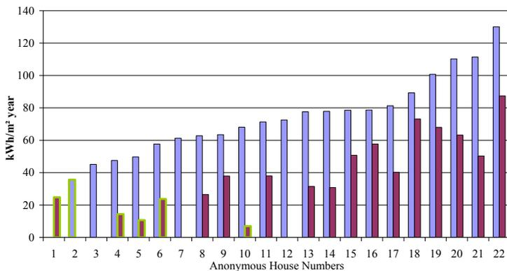
Figure 3 Electricity demand (ventilation, heating, DHW) according to BR08 low energy class 1 (blue), Net Space Heating demand (red) maximum prescribed demand 25 kWh/m<sup>2</sup> year
