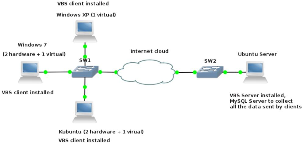
Figure 3.1: Topology of our testbed
