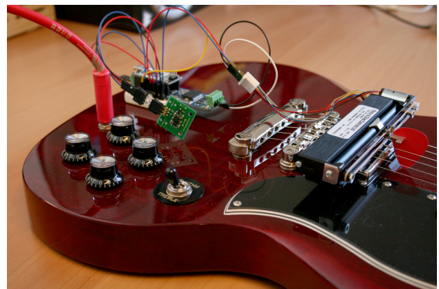
Figure 3. Implementation of the proof-of-concept guitar, which consists of an accelerometer, guitar, microcontroller, motor controller, motorized fader, and a pick.
