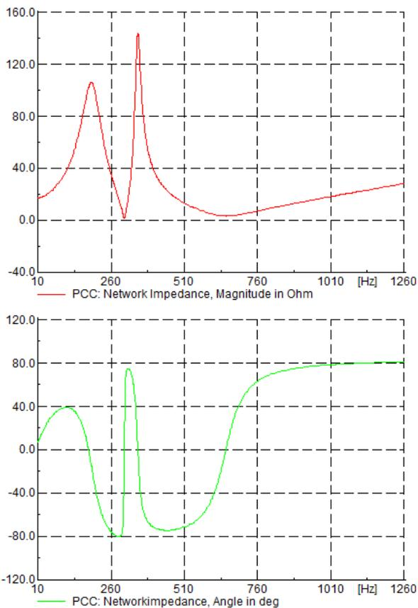
Fig. 9 Impedance plot in the point of common coupling from model with harmonic current source.
