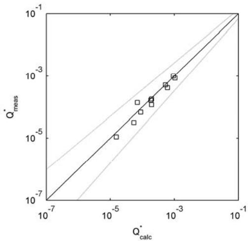
Figure 17: Evaluation of CLASH NN-Model against data by Lissev (1993).
