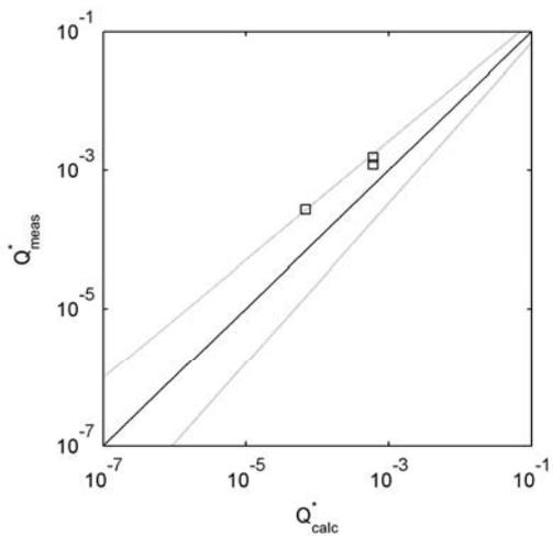
Figure 19: Evaluation of CLASH NN-Model against data by Kuhnen (2000).
