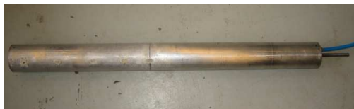
Figure 6: Picture of the test pile with an outer diameter of 80 mm. The cords are lead out through the blue cable.
