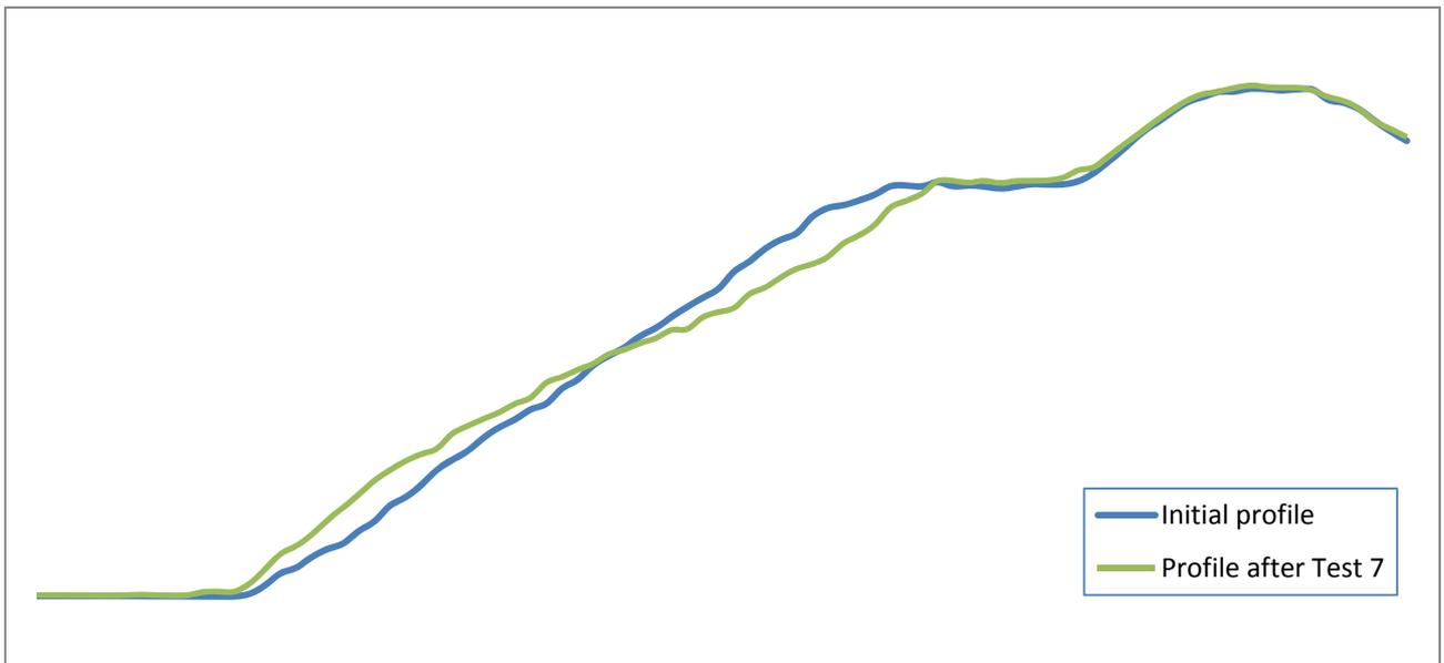
**Figure 45: Profile after test 7 ( $H_{m0} = 3.56$  m,  $T_p = 8$  s and WL = +2.4).**
