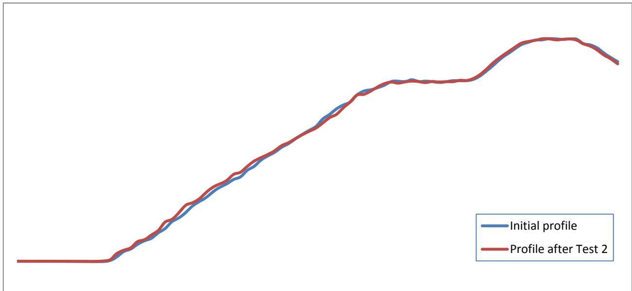
Figure 42: Profile after test 2 ( $H_{m0} = 3.17$  m,  $T_p = 8$  s and WL = +0.2 m).
