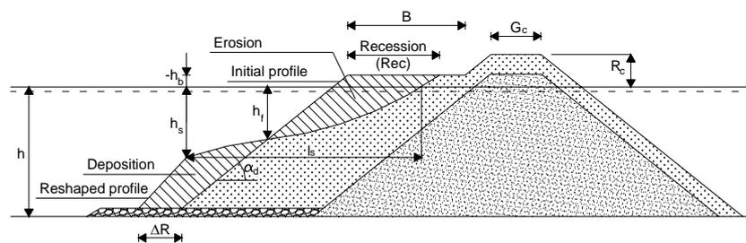
Figure 8: Definition of initial and reshaped profile parameters.
