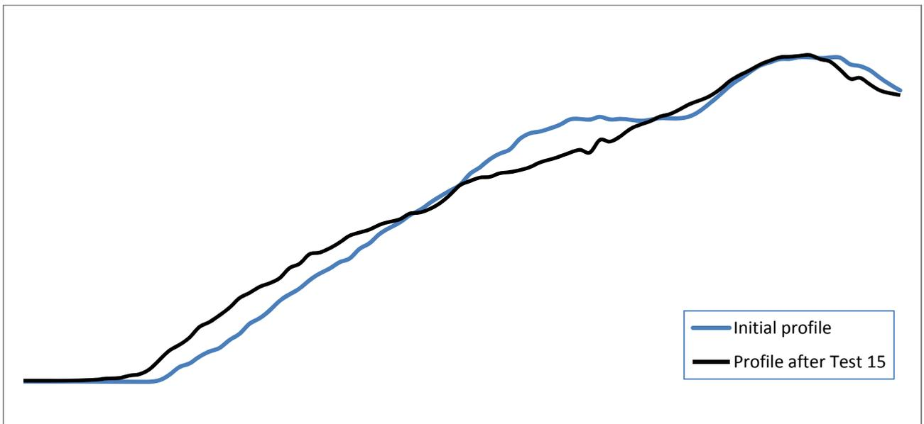
Figure 49: Profile after test 15 ( $H_{m0} = 4.61$ ,  $T_P = 11$  s and WL = +2.4).
