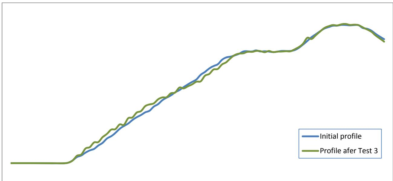
Figure 43: Profile after test 3 ( $H_{m0} = 4.05$  m,  $T_p = 8$  s and WL = +0.2 m).
