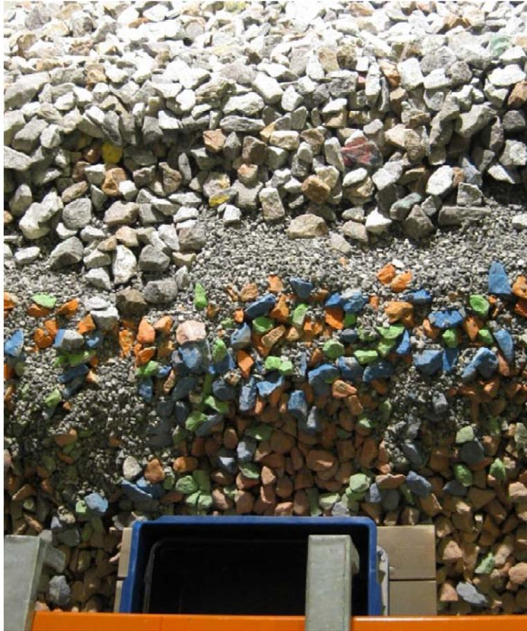
Figure 11: Damages to crest of structure after test 15.
