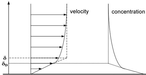
**Figure 1 Typical velocity profile for boundary layer flow**
