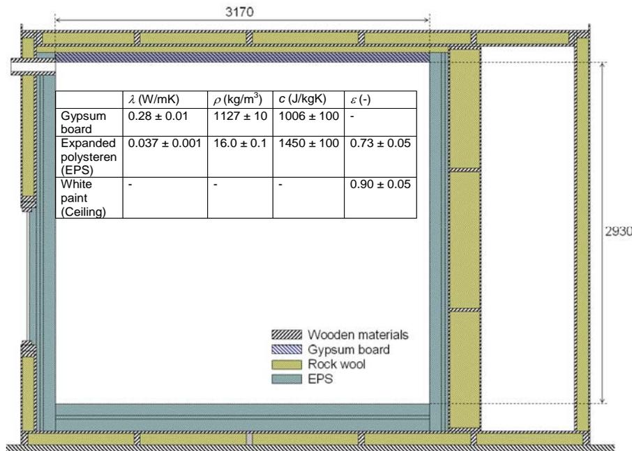
Figure 1. Vertical section of the test room.
