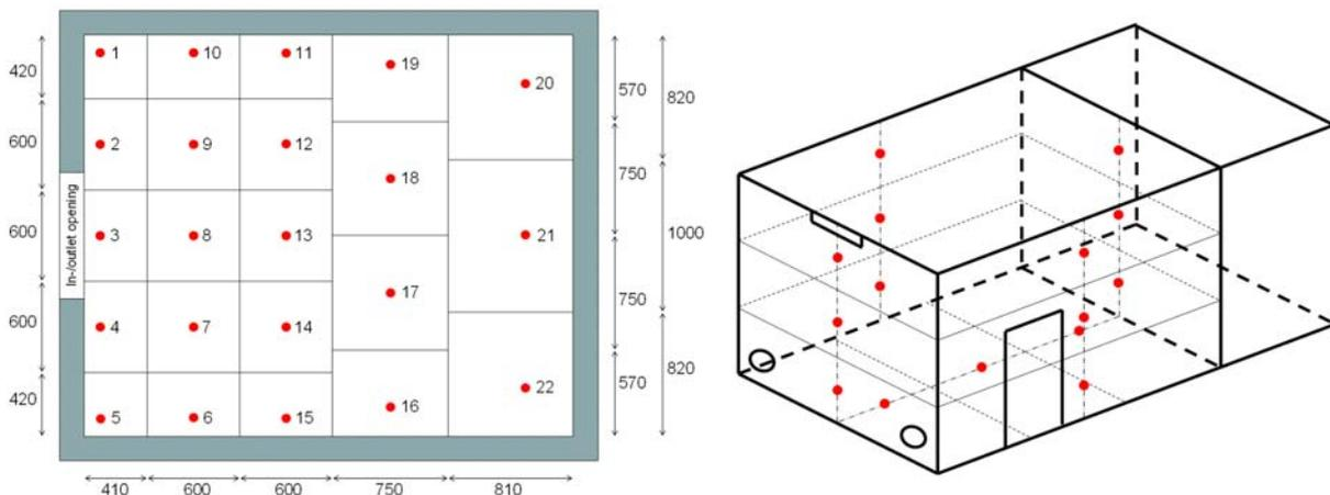
Figure 3. Left) Subdivision of the ceiling into 22 sections and location of sensors (top view), Right) Subdivision of the walls and the floor into 3 sections and location of sensors
