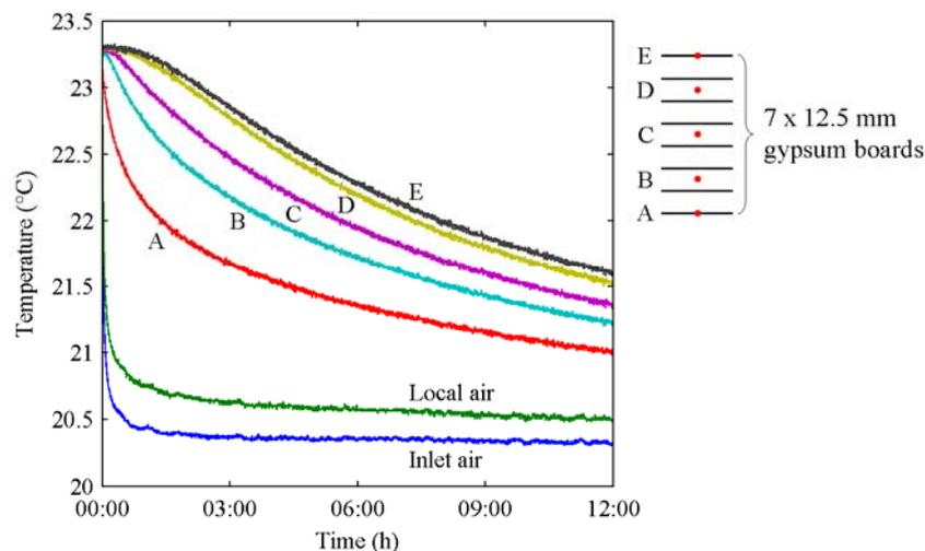
Figure 4. Temperatures measured at position 8 during an experiment with mixing ventilation with 6.7 ACH and an initial temperature difference of  $\Delta T_0 = 2.9$  K (A-E: different layers of the ceiling, A: internal surface, E: external surface).
