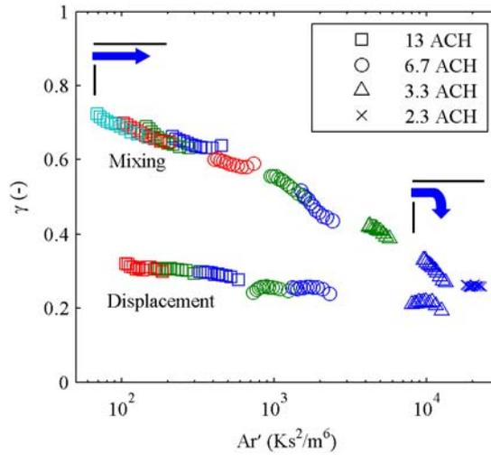
Figure 6. Ratio,  $\gamma$  of convective to total heat flow from the ceiling depending on  $Ar'$  for mixing and displacement ventilation; hourly values, first hour excluded; different colours relate to different experiments.
