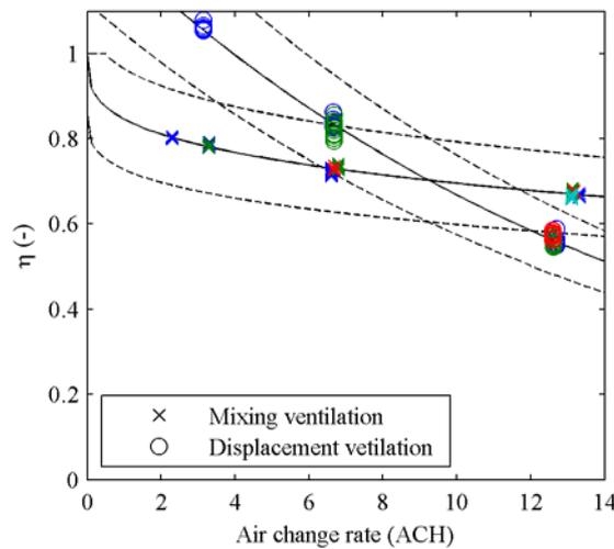
Figure 7. Temperature efficiency,  $\eta$ , depending on air change rate for mixing and displacement ventilation; hourly values, first hour excluded; different colours relate to different experiments. Fitted curves with estimated uncertainty bands ( $\pm 14\%$  [10]).
