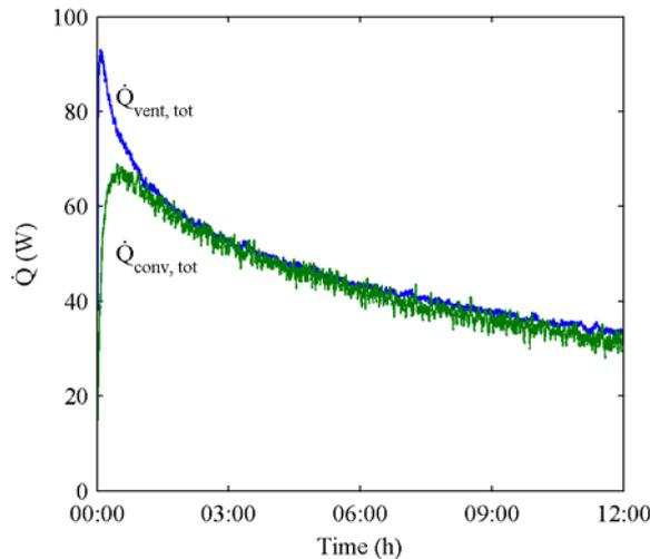
Figure 5. Total heat flow removed from the room obtained from direct measurements ( $\dot{Q}_{vent, tot}$ ) and from integrating the convective heat flows over all surfaces ( $\dot{Q}_{conv, tot}$ ) for an experiment with mixing ventilation,  $ACH = 6.7$  ACH,  $\Delta T_0 = 2.9$  K.
