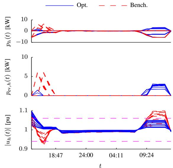
Fig. 8. Top: The total consumption in the optimized case (blue, solid), and the benchmark case (red, dashed). Middle: Corresponding EV charge schedule. Bottom: Resulting voltage profiles, as well as voltage limits (dashed, magenta).
