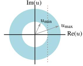
Fig. 2. Constraint for the voltage amplitude, where the shaded region visualizes the allowed range of  $u$ . The dashed line illustrates the approximated constraint for the lower limit.
