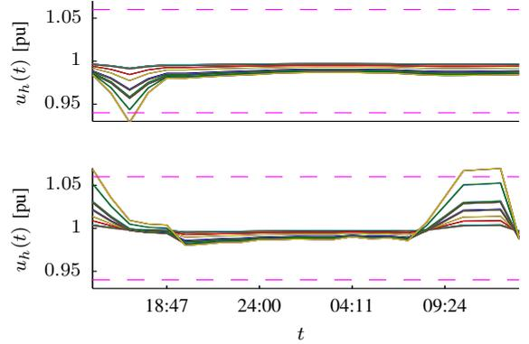
Fig. 6. Top: Voltage profile resulting each leaf by configuration 1 (solid), and allowed voltage range (dashed). Bottom: Similarly, voltage profiles by configuration 2.
