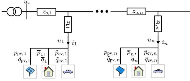
Fig. 1. Conceptual outline of a radial of the low-voltage grid, illustrating the consumers, with active and reactive solar production ( $p_{pv,i}$ ,  $q_{pv,i}$ ), EV consumption ( $p_{ev,i}$ ,  $q_{ev,i}$ ), and inflexible consumption ( $\bar{p}_i$ ,  $\bar{q}_i$ ).
