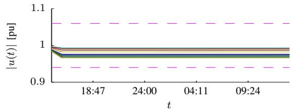
Fig. 7. Allowed voltage range (dashed), and resulting voltage profiles (solid), for the optimization based approach with  $H_{\text{ev}} = H$  and  $H_{\text{pv}} = \emptyset$ .
