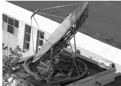
Fig.13. A solar parabolic dish thermal collector using the new MSS
