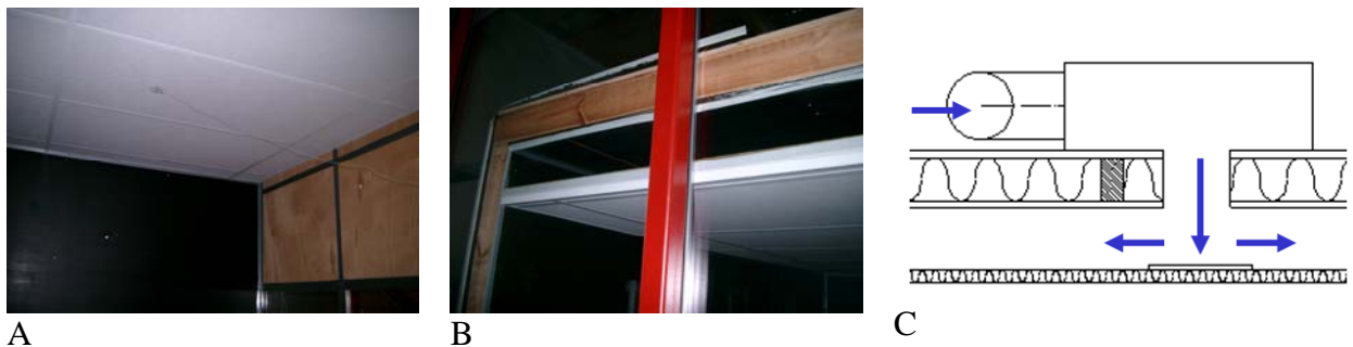
Figure 4. A: Test room with diffuse ceiling inlet. B: Location of acoustic ceiling below the ceiling. C: Supply opening to the plenum.
