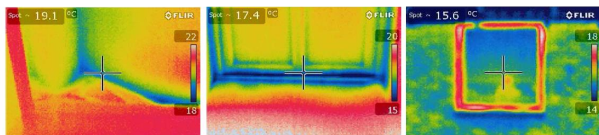
Figure 19: Thermal infrared images of the studied house (illustration of lack of airtightness, air leaks and thermal bridges)
