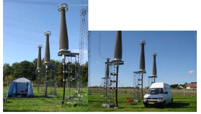
Fig. 5 Field test facilities at each cable end of the 400 kV cable system
