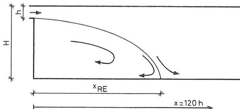
Figure 2. Sketch of backward facing step geometry.  $h/H = 1/6$ .
