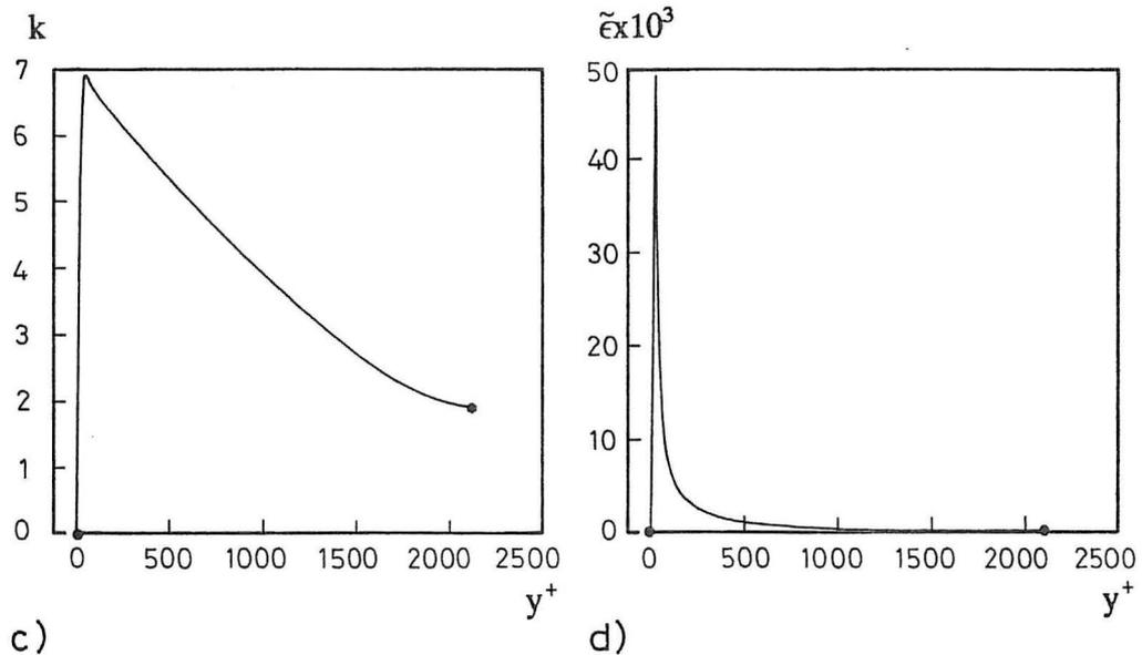
Figure 1. Simulated data from the straight channel flow (line). Experimental data by Laufer 1949 (plus). RSM data by Launder and Tselepedakis 1990 (square). a)  $U^+$  values as a function of  $y^+$ , b) shear stress profiles, c)  $k$  profiles and d)  $\tilde{\epsilon}$  profiles.
