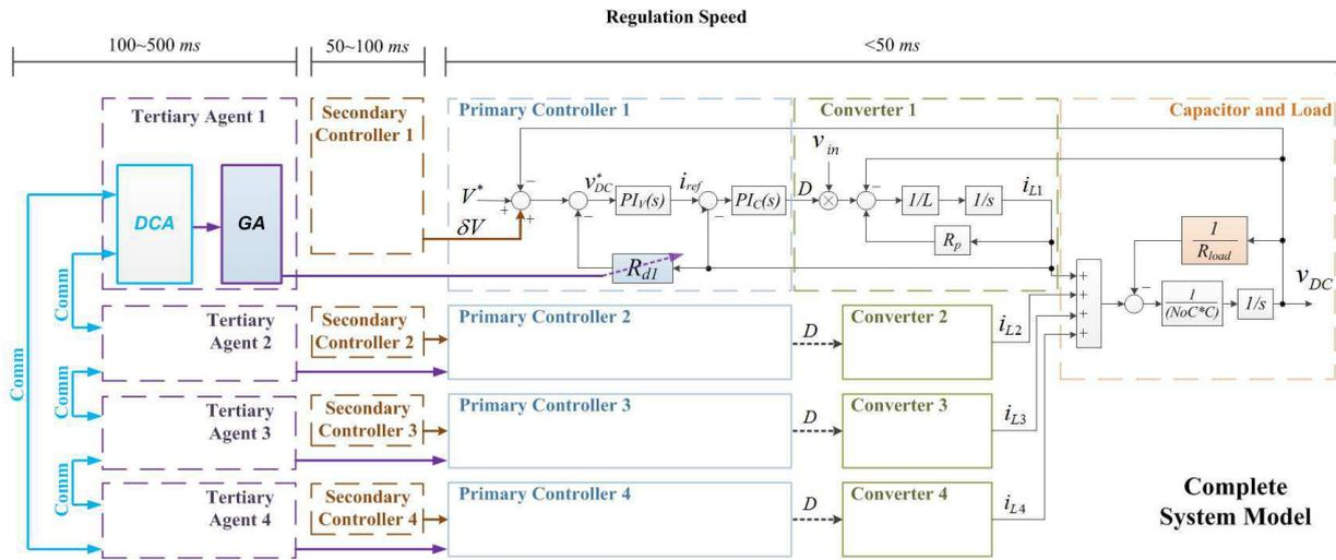
Fig. 4. Complete system model for HiL simulation.
