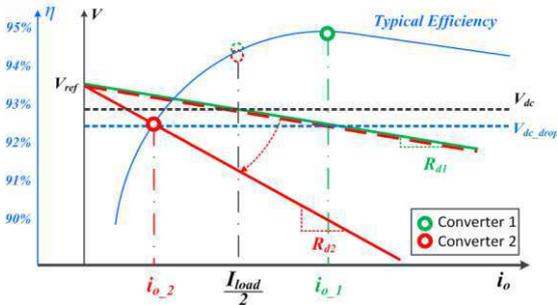
Fig. 3. Typical efficiency curve and adaptive VRs.
