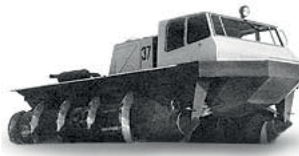
Figure 3. ZiL SHN-1, the screw-driven all-terrain vehicle, 1968 (image source: http://www.vsevezdehody.ru )
