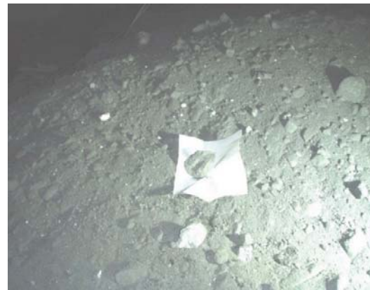
Figure 3: Fragmentation for double-primer placement AL992. The size of the paper is A4.
