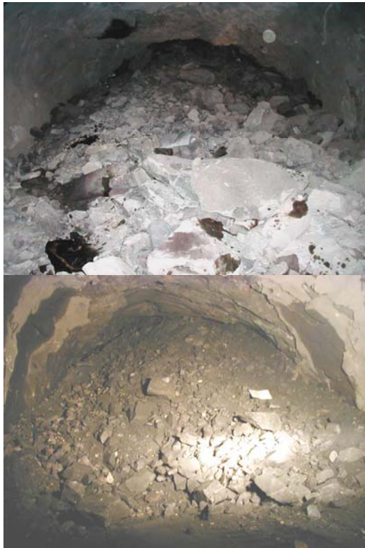
Figure 2: Comparison of fragmentation in ordinary ring with lowest primer (upper) and test ring with middle primer (lower). The paper in both pictures is the same paper with a size of 400x500 mm (Zhang, 2005).
