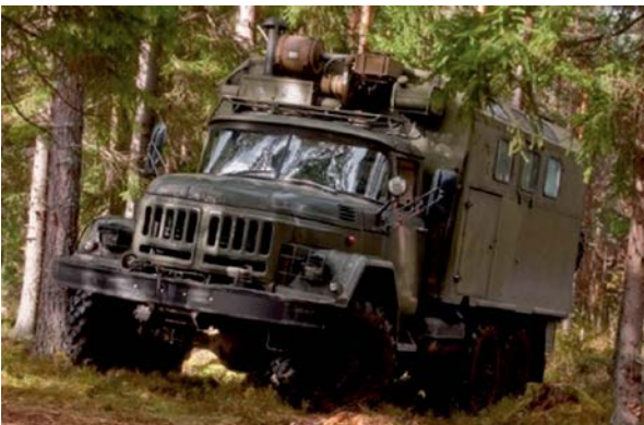
Figure 4. ZiL-131NS, the northern modification of a standard production model, 1986 (image source: Wikimedia Commons)
