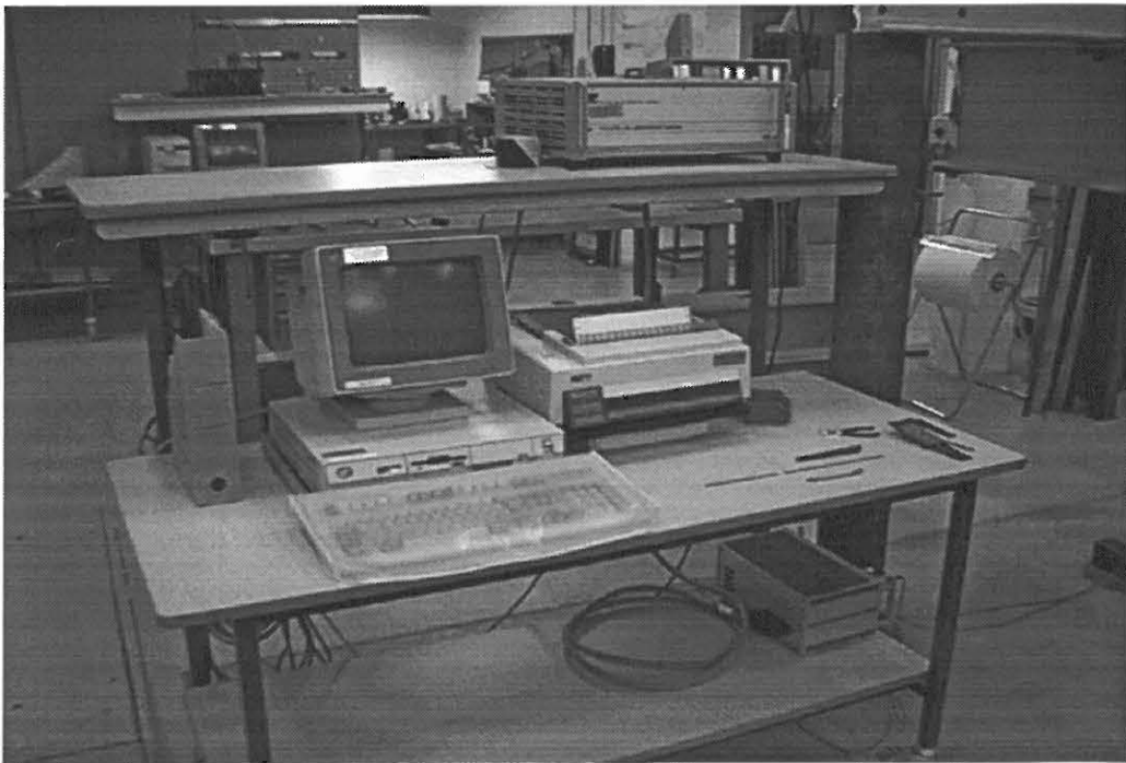
Figure A.9: Photo of the data acquisition system used for the static tests of parts of the structure.
