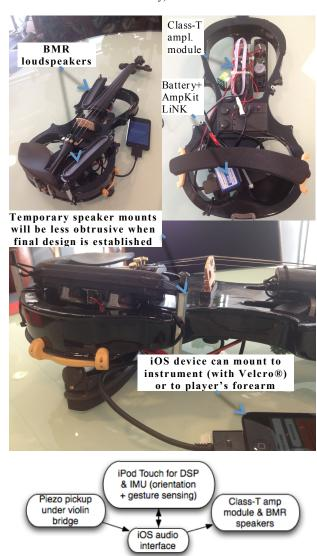
Figure 1. Components of the hybrid violin platform. *Top left*, front view of loudspeakers. *Top right*, rear view of amplifier module, battery & iOS audio interface. *Middle*, side view close-up. *Bottom*, audio flow diagram.
