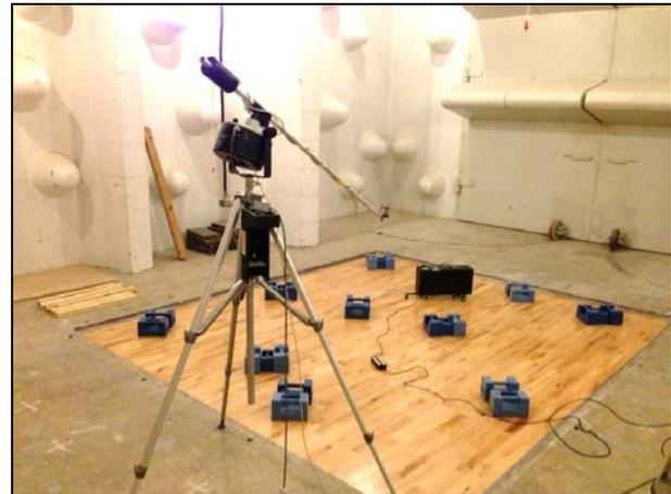
Figure 3. Test setup for laboratory measurements of impact sound improvement. The photo shows the standardized tapping machine and the floor load 25 kg/m<sup>2</sup>.
