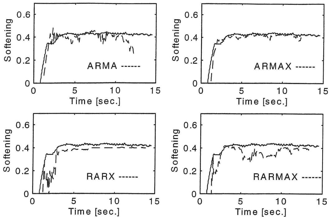
Figure 4: The estimated softening as a function of time. Earthquake = 0.3 g.
