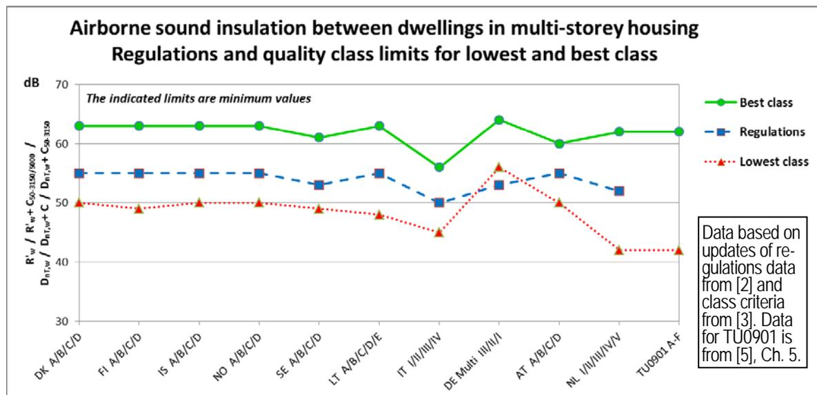
Figure 2 – Airborne sound insulation limits for highest and lowest classes in 10 classification schemes in Europe and regulatory requirements for the same countries. TU0901 class limits for highest and lowest class shown in the right side for comparison. Note: The diversity of descriptors appears from the Y-axis label. The graphs present the numbers only. No conversions between descriptors have been applied.
