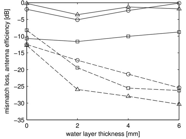
Fig. 4. Mismatch loss (solid line) and antenna efficiency (dashed line) as functions of thickness of the water layer. Pavement properties:  $\epsilon_r = 6$ ,  $\sigma = 10^{-4}$ . ( $\circ$  ... dipole,  $\triangle$  ... meander dipole,  $\square$  ... patch)
