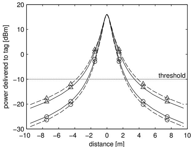
Fig. 11. Power delivered to the RFID tag on the road versus distance of the reader. (Pavement permittivity: solid line  $\epsilon_r = 6$ , dashed line  $\epsilon_r = 12$ ; Polarization:  $\Delta$  ... vertical,  $\circ$  ... horizontal)
