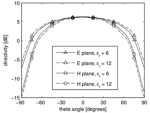
Fig. 5. Radiation patterns of the planar dipole antenna.
