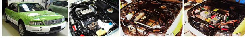
Fig. 5: AAUDI prototype. Views of the engine compartment: original Audi A8 4.2 Quattro (second), empty (third) and after conversion into AAUDI (forth).
