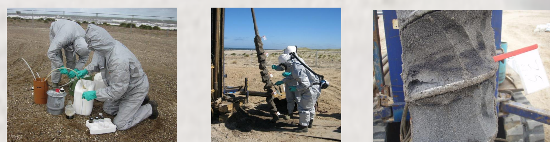
Fig. 3: Sampling of site water and soil with visible DNAPL. Over 2½ years, more than 2000 water samples and 1200 soil samples were analyzed in NorthPestClean.
