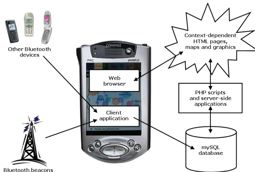
Figure 3. Just-for-Us prototype system architecture
