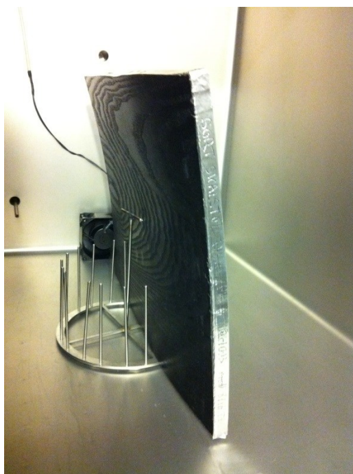
FIGURE 1. KITCHEN FRONT DOOR, CUT TO SIZE AND WITH SEALED EDGES, IN A 0.225 \text{ M}^3 CHAMBER.
