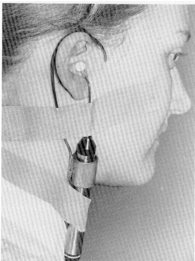
Fig. 3. Probe microphone mounted on subject to measure blocked ear canal pressure P_5 .
