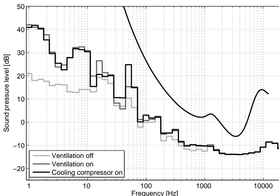
**Figure 6: Background noise measured in 1/3-octave bands in the listening position with ventilation off (light grey), ventilation on (dark grey) and ventilation and cooling compressor on (black). The black curve is the normal hearing threshold. The measured 1/3-octave bands from approx. 2 kHz and upwards is the noise floor of the measurement system.**
