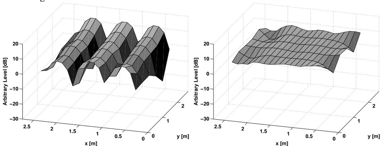
**Figure 4: Sound pressure distribution at 250 Hz in a horizontal plane at a height of 1.35m without (left) and with (right) sound field control. With sound field control it is only the regions close to the loudspeakers that exhibit significant pressure variations.**
