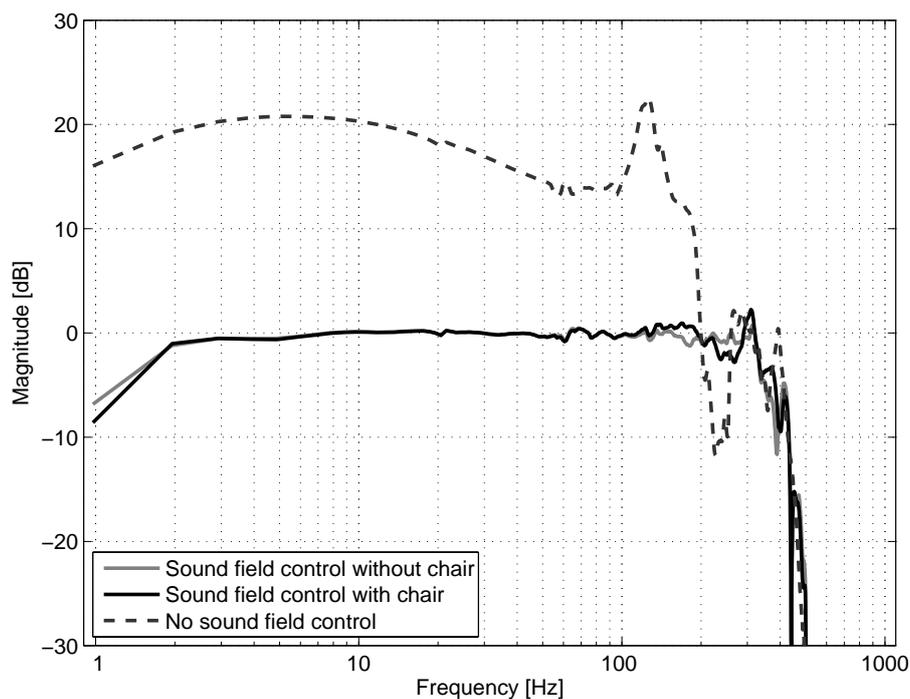
**Figure 5: Frequency response of the playback system in the listening position with sound field control and chair (solid black), with sound field control and no chair (solid grey) and without sound field control and with chair (dashed black). The deviations below 2 Hz is caused by low signal-to-noise ratio for this frequency area.**
