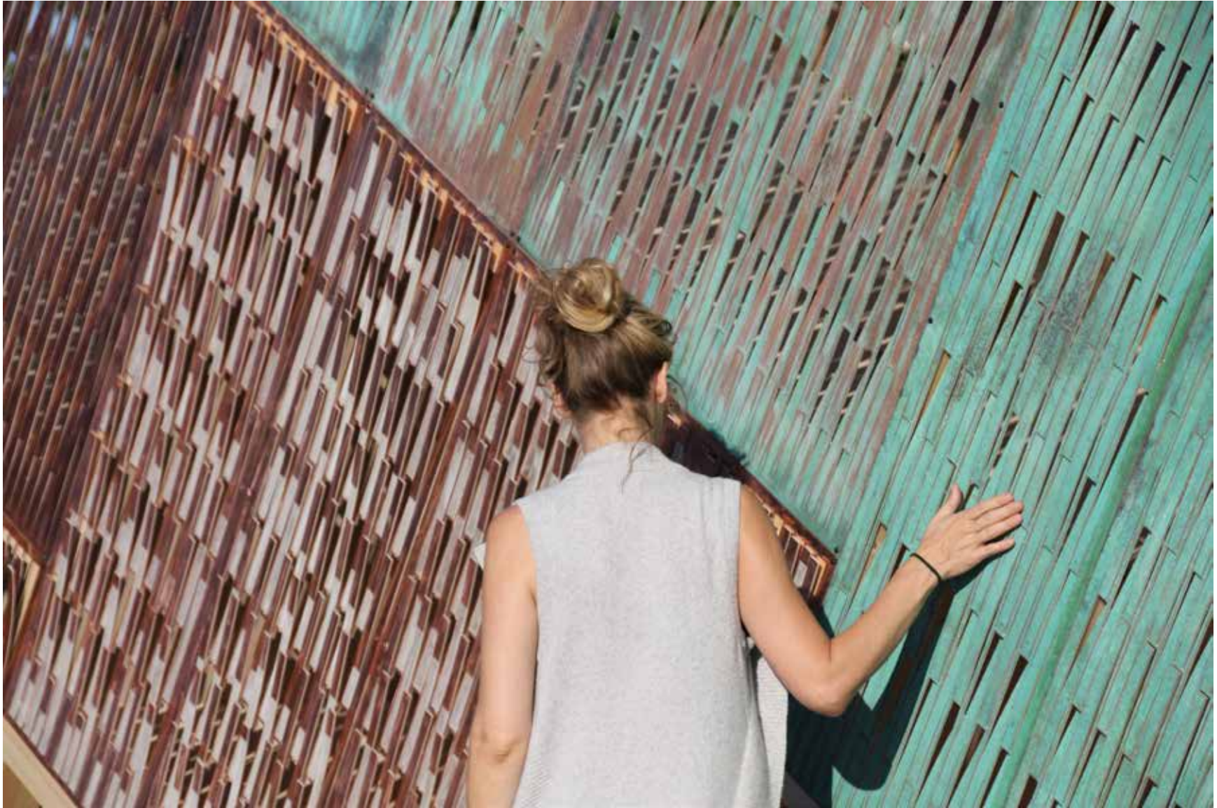
Figure 6. Full-scale prototype, measuring approximately three by eight meters as installed next to the Danish Architecture Centre, Copenhagen, for two months, for demonstration, measuring and observation. The image illustrates the articulation of the composite and its resultant bending behaviour. Photo by Isak Worre Foged.
