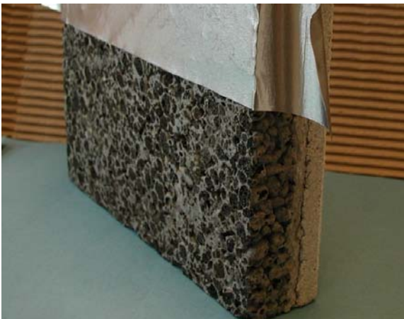
Light weight aggregate concrete with stucco
