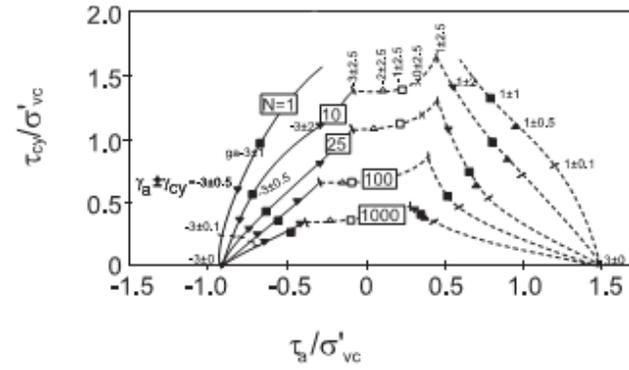
Fig. 7 Original Andersen's chart for undrained soil response (normalized by drained confining pressure)
