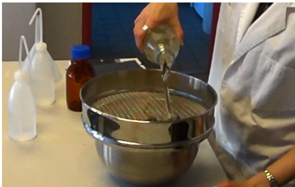
Figure 24: Unfiltered water samples are poured into a metal bowl through a 4mm sieve.
