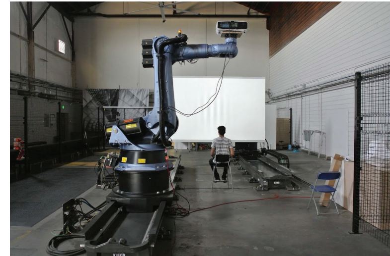
FIGURE 2: THE APPARATUS USED BY GEPSHTEIN, MCDOWELL & LYNN. LARGE INDUSTRIAL ROBOTS, CARRYING A PROJECTOR AND A SCREEN, WERE DEPLOYED TO MAP SOLID REGIONS OF VISIBILITY FOR STATIC AND DYNAMIC VISUAL PATTERNS ON THE SCALE OF ARCHITECTURAL DESIGN [2, 5].
