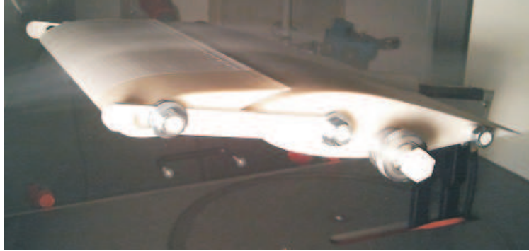
Figure 3.6 DU06-W200 double-element airfoil in the wind tunnel
