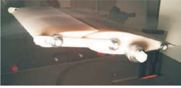
Figure 2. Double element airfoil in wind tunnel. (This figure is available in colour online.)
