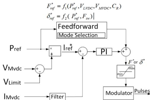
Fig. 4 Controller structure
