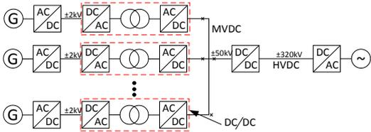
Fig. 1 DC Wind farm diagram
